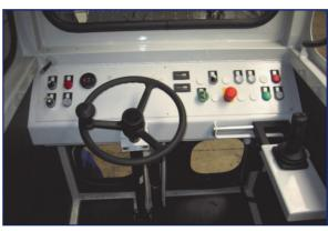
The GT can be easily moved by joystick and steering wheel
